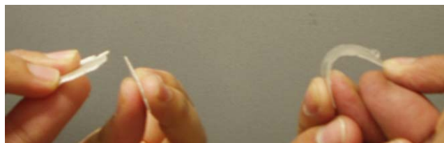
Figure 5. The increasing brittleness of the electrospun PLA/NCC composites with increasing NCC content [Left: 5% NCC; Right: 0.5% NCC]. [Color figure can be viewed in the online issue, which is available at wileyonlinelibrary.com .]
