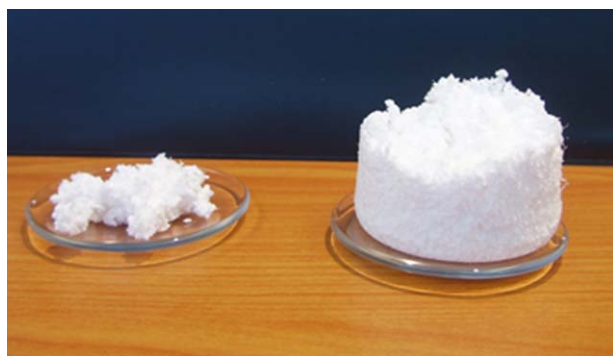
Figure 3. Photos of freeze dried 0% NCC electrospun PLA/NCC composite sample (left) and freeze dried 1% NCC electrospun PLA/NCC composite sample (right). [Color figure can be viewed in the online issue, which is available at wileyonlinelibrary.com .]
